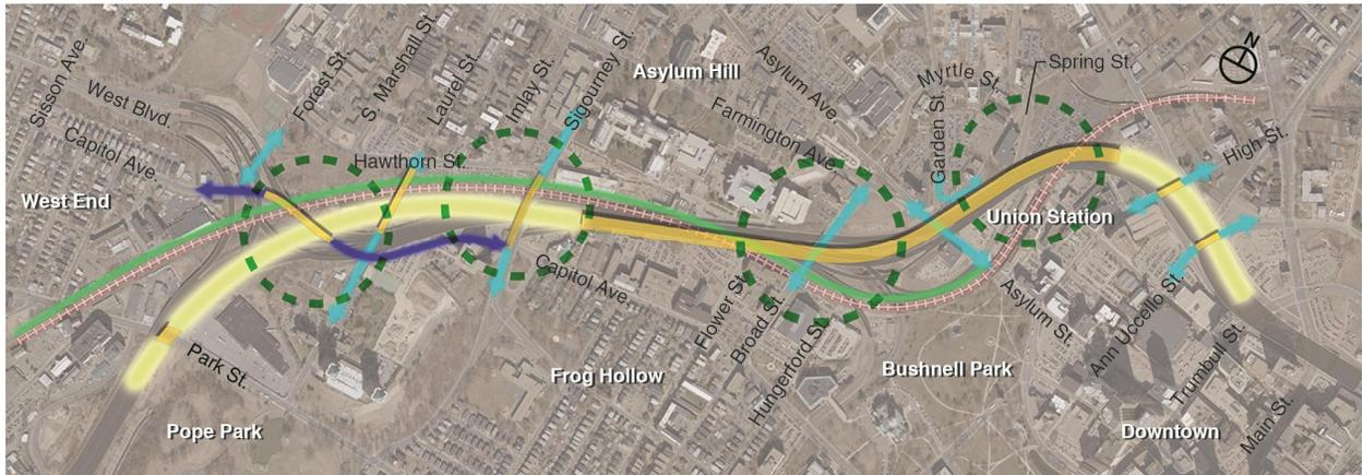
In this alternative, a new elevated highway would replace the existing viaducts with a single viaduct between Sigourney and High Streets. The new viaduct would be higher than the existing viaduct to provide minimum required vertical clearances over the railroad and local streets.
