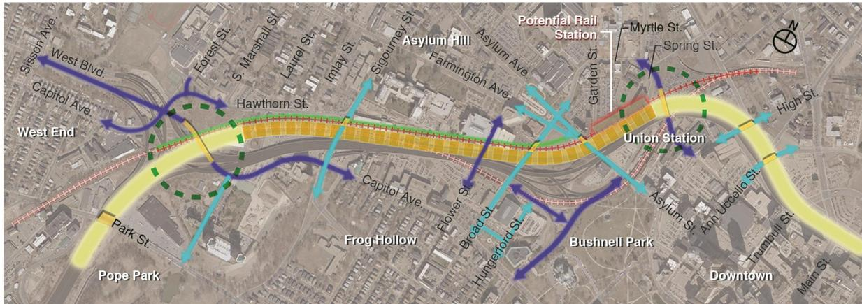
In this alternative, the railroad would again be relocated to the north of the highway to allow I-84 to be lowered below grade from Myrtle Street to Laurel Street in a tunnel.
